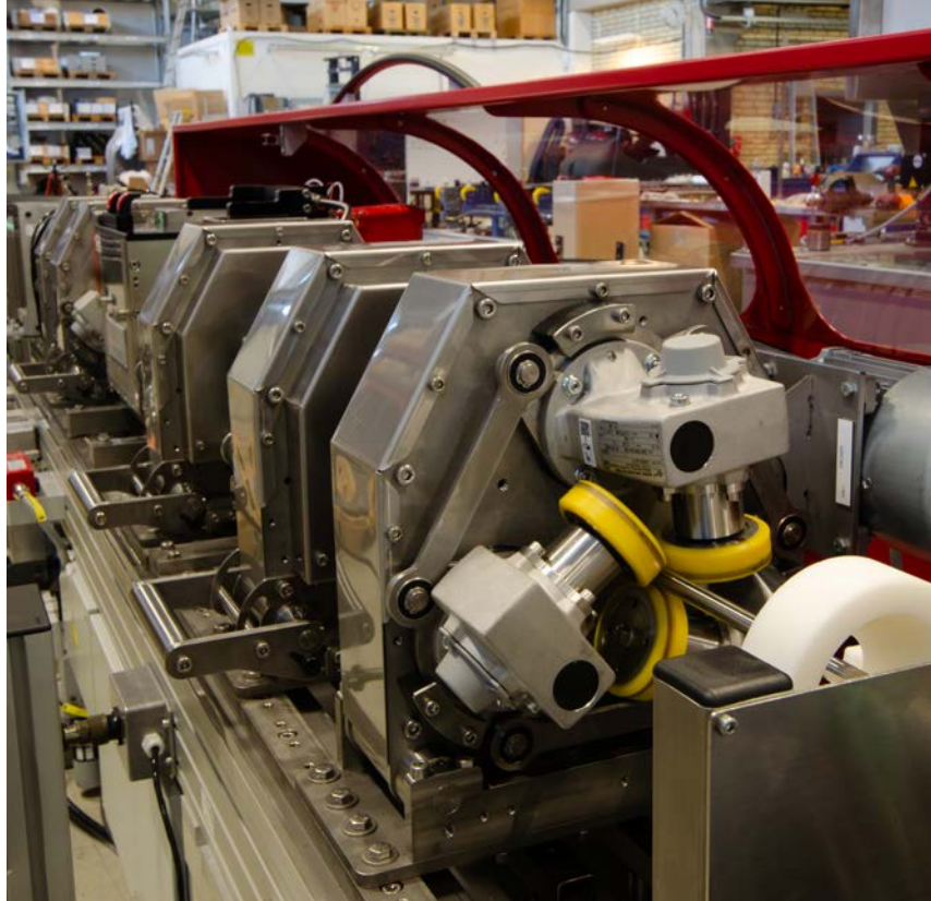
A close up of the triple pinch system which is adjustable for height and diameter of test product.
