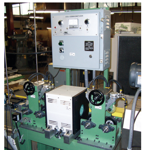
475 Demagnetizer and electronics on a "V" Roll Guide bench
