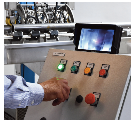
The remote operator station contains essential controls including the video monitor for checking transducer positioning with respect to the weldzone.
