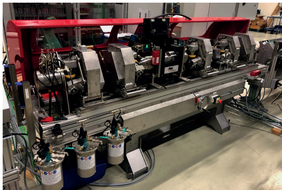
Figure 3: Picture of an Echomac® UT-25mm rotary system that includes an Eddy Current mounted encircling test coil. The Rotary UT inspection line is capable of inspecting the material passing through it in up to 8 directions of interrogation. It can test for internal (Normal incidence), CW Shear, CCW Shear, Transverse FWD, Transverse REV, and more. This NDT system can test bars or tubes.
