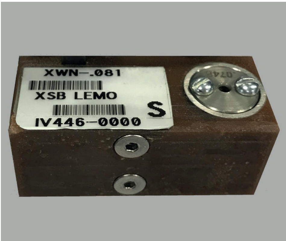
Figure 1: Eddy Current Wiretester Coil with inset guide bushing for testing small diameter wire.
