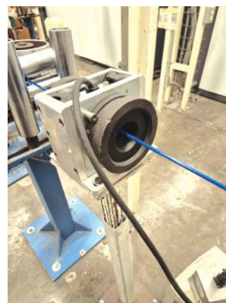
MAC® CP 65NS with bushing is shown testing single wire cable.
