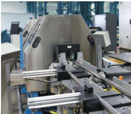
At input, bars enter through a demagnetizer before eddy current testing. On the left, a sample bar is held in the calibration station where it can be automatically fed through the testers when needed.
