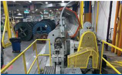
30" Syncro 7W Tubular Strander TBR228
