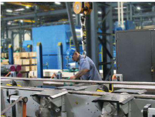
RGM® Operator prepares bundle of pre-aligned bars for transfer after testing.
