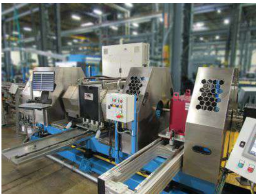
The system includes MAC Rotomac® and Echomac® test rotaries that detect surface defects and internal flaws. The slides in the foreground allow easy access for maintenance of the rotaries.
