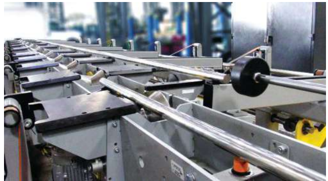
MAC's Aligner ensures the accepted bar ends are lined up for easy bundling.
