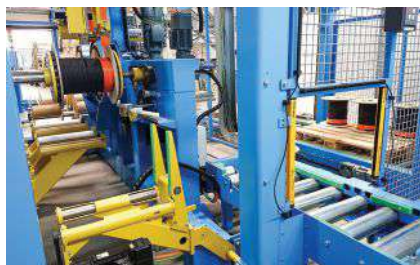
Winding and tapping stations, conveyor and palletizer...78
