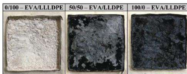
Figure 11. Residues of EVA/LLDPE blends filled with 60% MDH from cone calorimeter testing.
