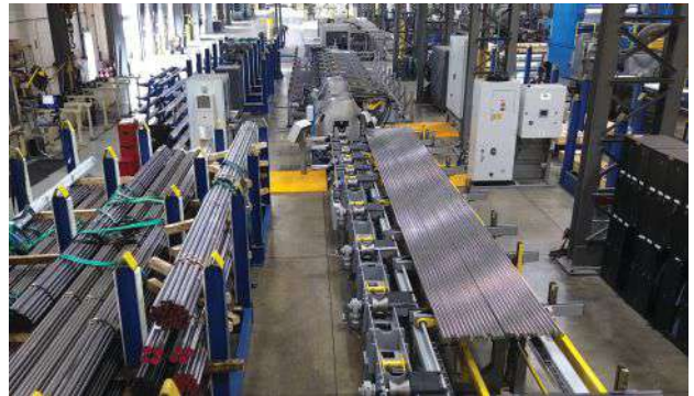
Bird's eye view of MAC®'s 105 ft, ultrasonic and eddy current equipped NDT system with automated materials handling at RGM®'s Illinois plant.
