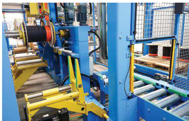
Winding stations and taping station (left), roller conveyor for ejection of faulty spools and palletizer (back). Images: © KURRE Systems
