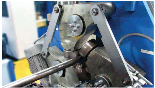
The “heart-of-the-system” triple pinch controls the entrance and exit of the bar as it passes through the test. This signature feature eliminates vibrations that can cause false rejects, saving time and labor.
